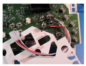
The F150 instrument cluster Hot in Start & Run power is the RD/LG wire and the Hot in Run power is the GY/YE wire.
