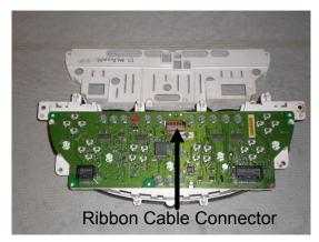
Unplug the ribbon cable connector and remove the Printed Circuit Board (PCB) from the back of the cluster. Locate the male pins on the back of the oil pressure gauge (bottom left gauge when viewed from the back of the cluster.)
